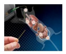
The small sensors, at 300, 640 and 1000 micron diameters and pressure ranges of +/- 300 mmHg and 0-10 bar, are designed to be used in any pre-clinical physiological pressure measurement application.
