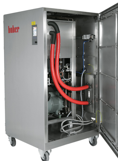
Figure 15: Ex-p Pressurised cabinet for use within hazardous areas in ATEX zones 1 & 2.
