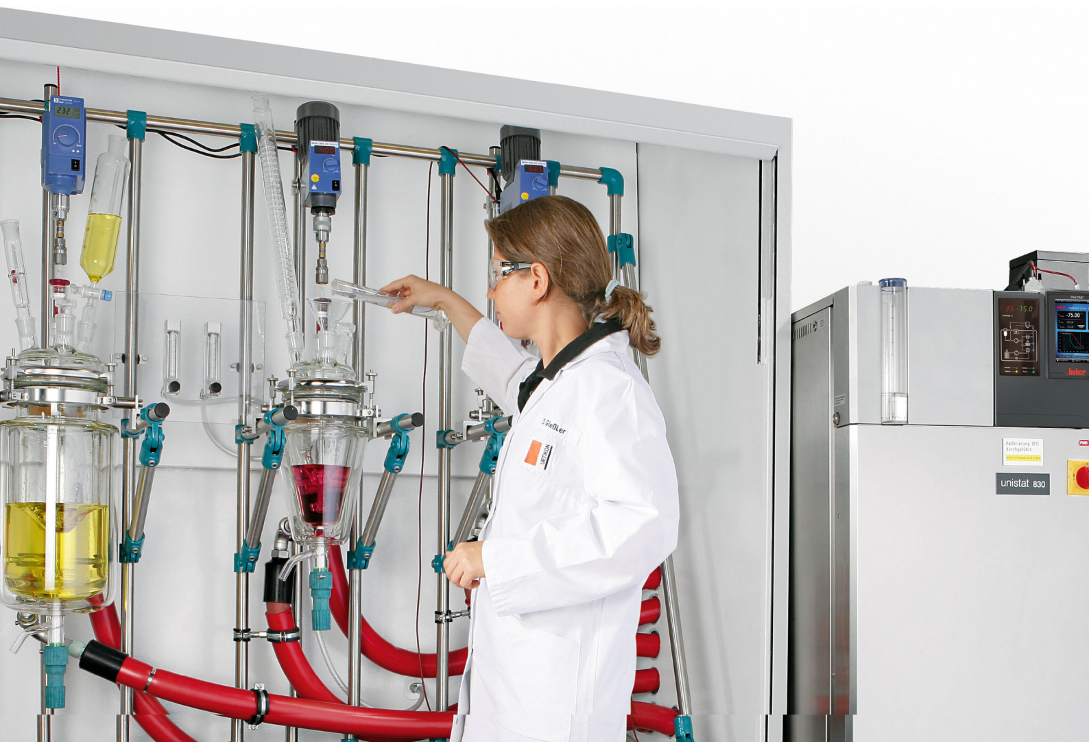
Figure 5: Unistats are in use in many industries, particularly in reactor temperature control.
