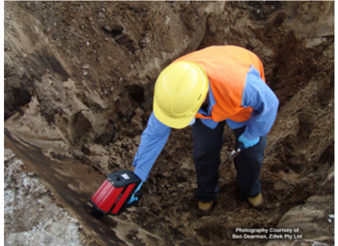
Figure 1 - A2 FTIR analyzer with diffuse reflectance sampling interface rapidly records the molecular spectrum of the sample with no preparation required.
